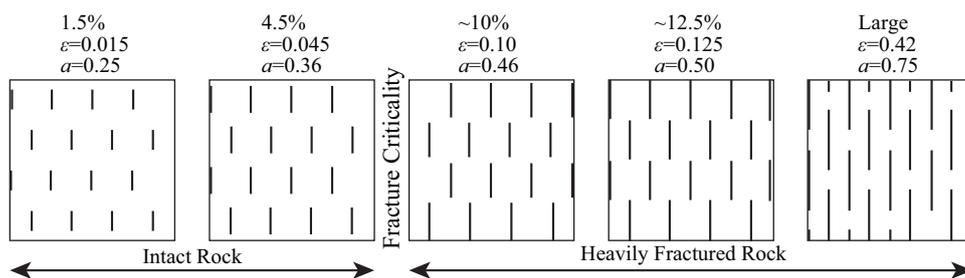
**Figure 2.** Schematic illustration of uniform cross-sections of three-dimensional distributions of penny-shaped microcracks for five percentages of shear-wave velocity-anisotropy (%SWVA). Above each distribution are listed: %SWVA;  $\epsilon$ , crack-density; and  $a$ , crack radius in a unit cube. Fracture-criticality is indicated at  $\sim 5\%$ SWVA.
