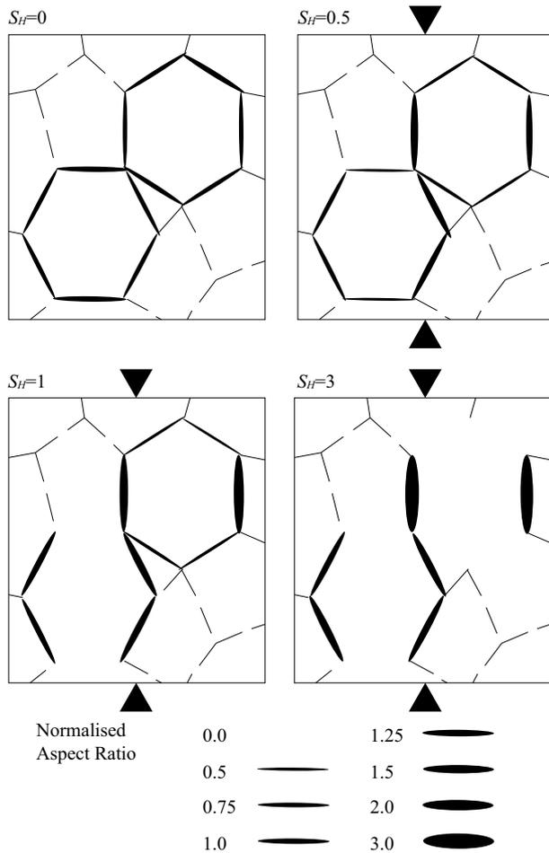
**Figure 3.** Schematic illustration of deformation of microcracked rock by Anisotropic Poro-Elastic (APE). Horizontal cross-section of an initially random distribution of fluid-saturated vertical microcracks deformed by four values of horizontal differential stress,  $S_H = 0, 0.5, 1.0, 3.0$ . Behaviour described in text.
