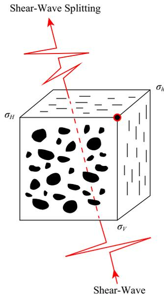
**Figure 1.** Schematic illustration of shear-wave splitting in stress-aligned microcracked rock, where  $\sigma_H$ ,  $\sigma_h$ , and  $\sigma_V$  are the maximum-horizontal, minimum-horizontal, and vertical stresses, respectively.
